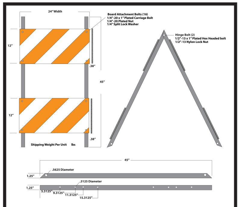
14 Gauge Galvanized Plated Steel Leg Specially Formulated ABS Plastc Board, Fluted for Superior Strength Inside of Bottom Board Can be Stenciled or Digitally Printed with Customers Name or Full Color Logo Boards Require NO Special Treating for Sheeting or Ink Adhesion
